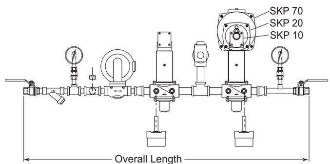
When using the Siemens SKP20 and SKP70 actuators for pressure regulating and ratio regulating functions, the sensing piping is not included. For proper operation, the sensing pipe should be at least 1/4" I.D. and connected a minimum of 5 pipe diameters downstream in a non-turbulent area.
